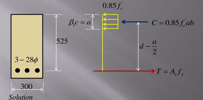
Calculate tensile and compressive forces T and C:
